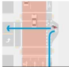
T-Intersection "Jughandle" Sidewalk Configuration
